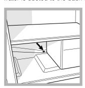
discharge outlet (see diagram) where the heat produced by the compressor causes it to evaporate. It is necessary to clean the discharge hole regularly so that the water can flow out easily.
